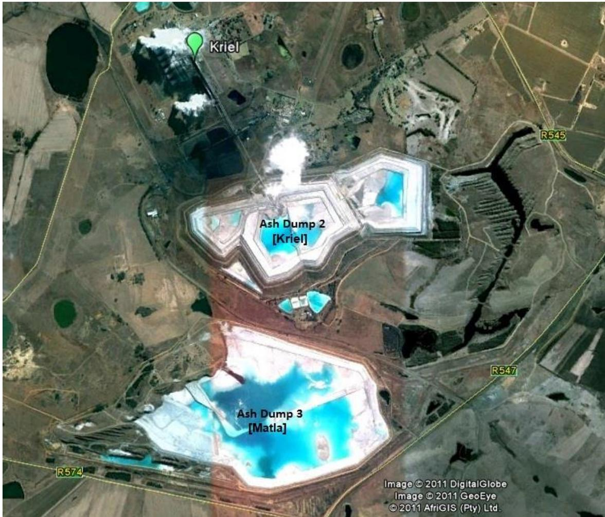
Figure 3-9: Existing ash disposal facilities near the Kriel Power Station
